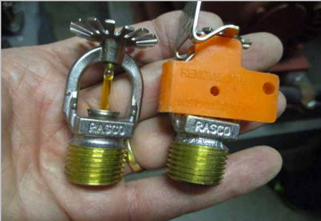
Rasco sprinkler heads.
