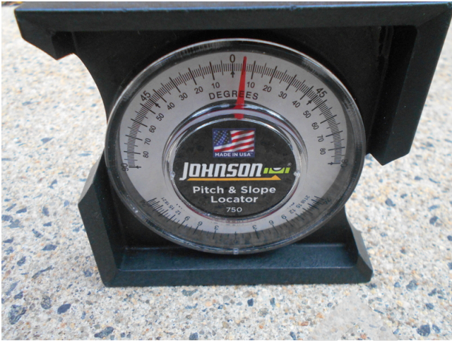
9. Leasing office handicap ramp slope 2, compliant
