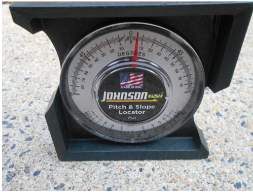
Leasing office handicap ramp slope 2, compliant
